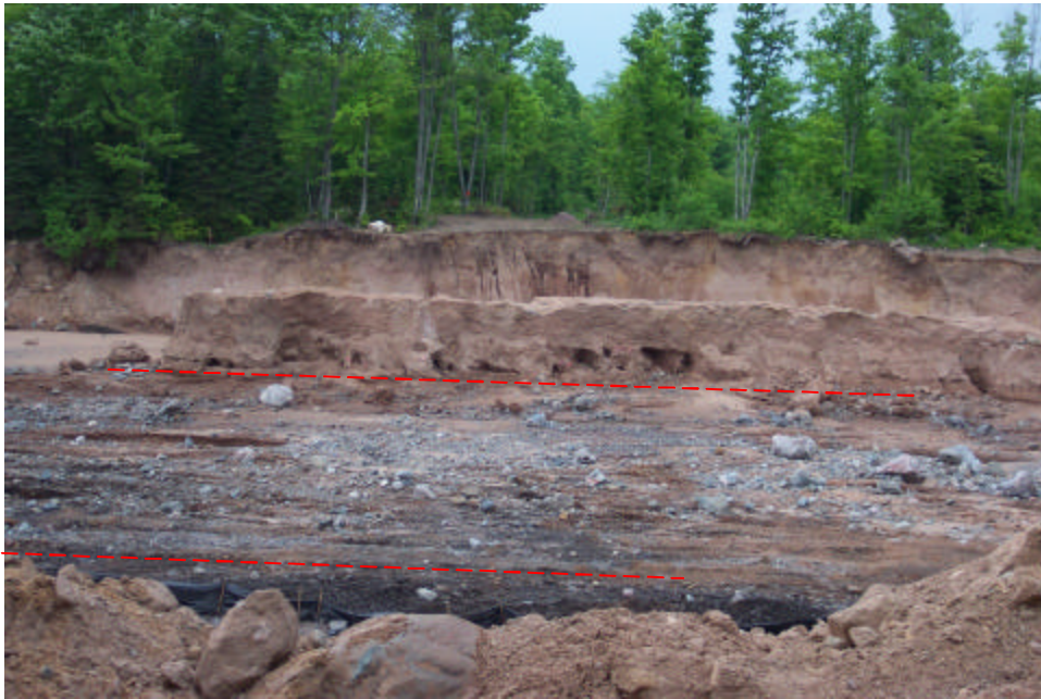
Figure 8 Overall stratigraphy of the area. Note the light-brown, dry SP-SM unit on the far channel wall and erosional remnant within the channel (above upper red line), the dark-brown, moist to wet finely bedded SP unit below the SP-SM unit (between the red lines), and the black organic silt (OL) unit at the base (below lower red line). View is from the right channel wall looking to the left directly along the alignment of the former fuse plug.
