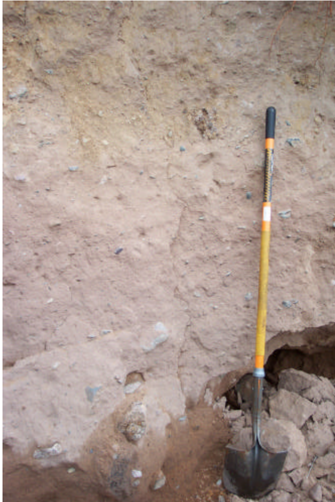
Figure 2 Detail of "Coarse-textured glacial till." This material is generally 90% fine to coarse sand and 10% non-plastic fines (SP-SM), with occasional gravel, cobbles and boulders. Note that some faint stratification is present. The stratification and coarse-grained material point to a higher-energy glacial environment, possibly originating closer toward the ice terminus. View is of left channel downstream of former fuse plug.
