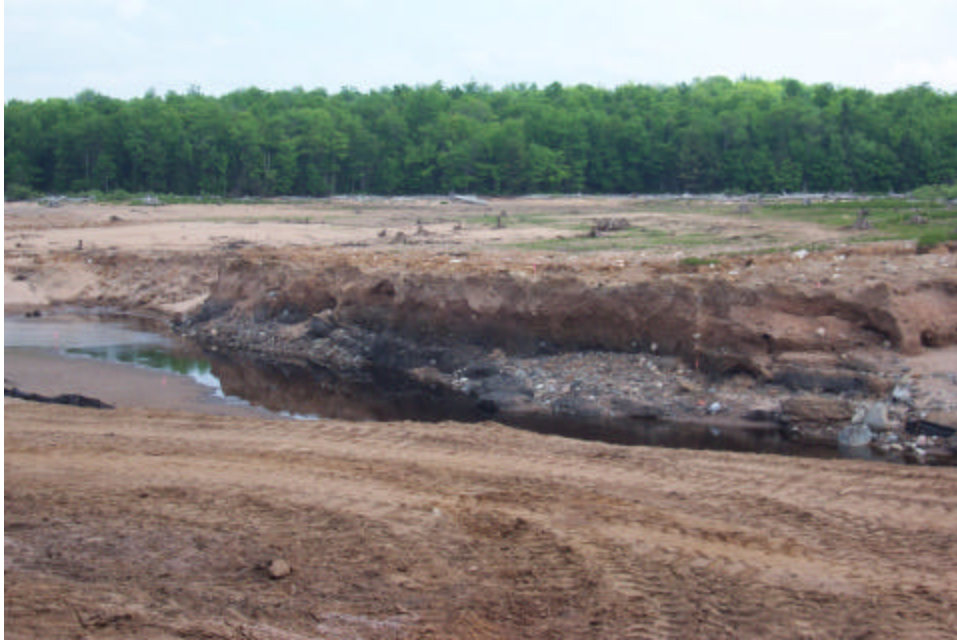
Figure 7 Note the dark gray to black unit stratigraphically below the "Coarse-textured glacial till." This deposit appears to be an organic silt (OL) with a very high dry strength and contains a significant fibrous organic content. View is of left channel upstream of former fuse plug.
