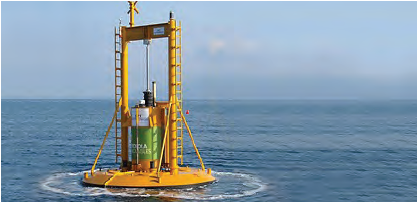
Experimental Point Absorber Wave Energy Device
