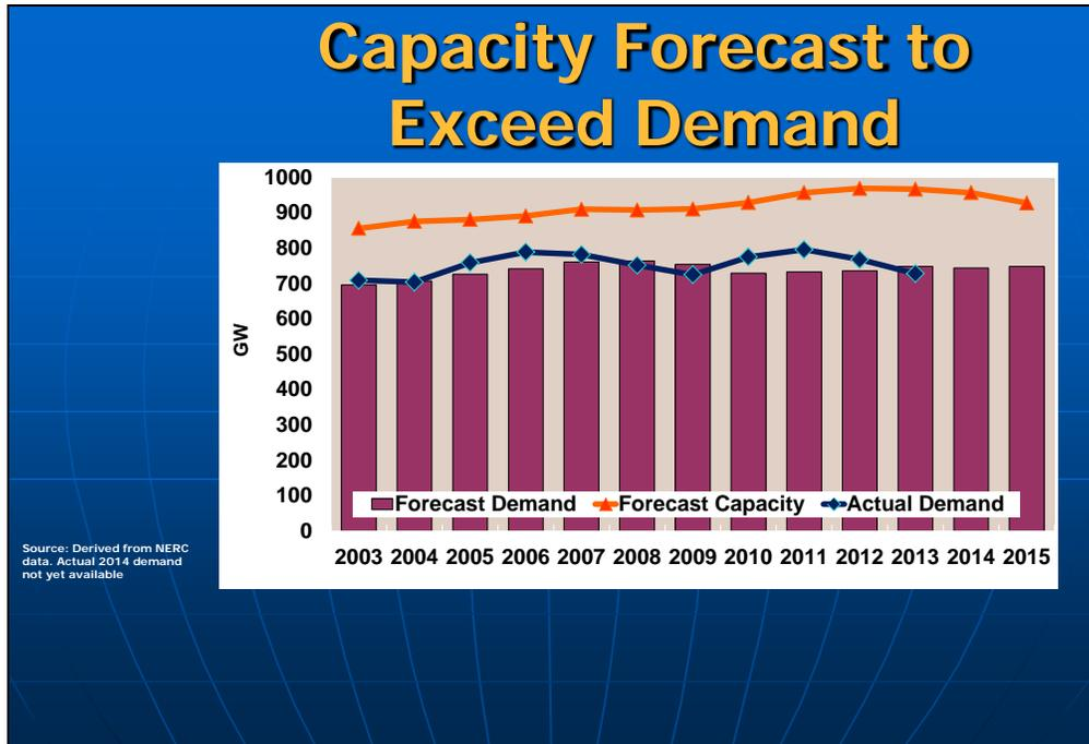
EIA has forecast a 2.9 percent increase in electric demand from 2014, reflecting an expected return to more typical conditions from last year’s unusually mild weather. This compares to a weather adjusted increase of approximately 1 percent over last year’s forecast. This growth is driven primarily by the commercial and industrial sectors, as opposed to the residential sector, which is a reversal from the past few years.
