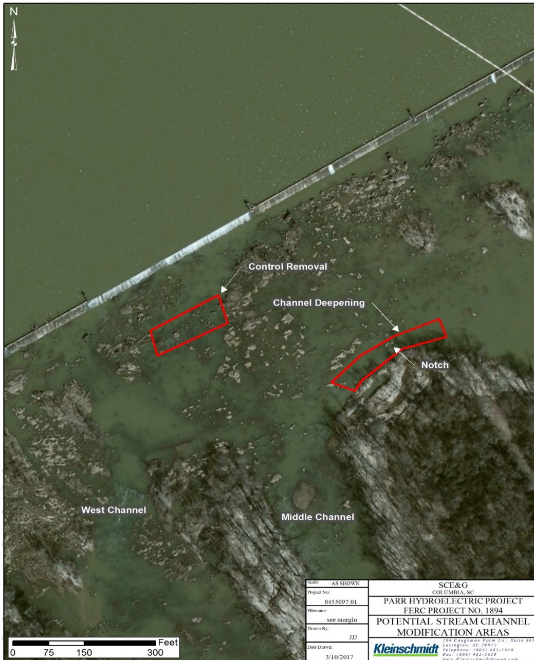
Figure 3-12. Potential areas for channel modification in the West Channel of the Broad River (Source: Dominion Energy, 2018b; Exhibit E-4 Water Resources – Adaptive Management Plan for Enhancements to the West Channel Downstream from Parr Shoals Dam).
