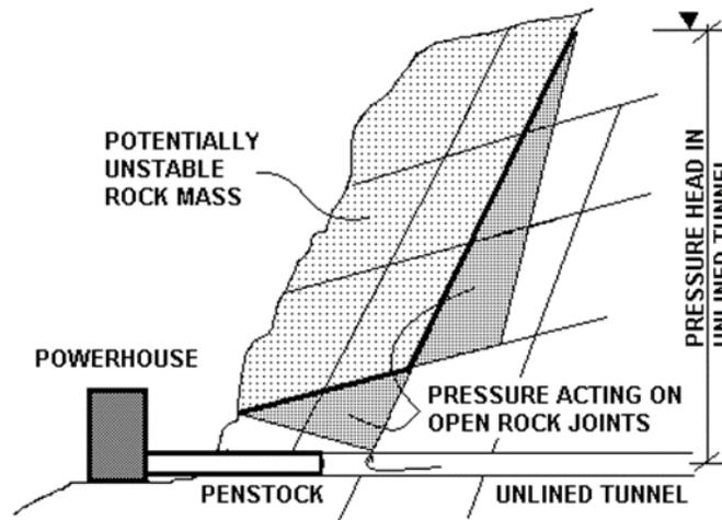
Fig. 19. Diagram of rock wedge at Schoellkopf.
