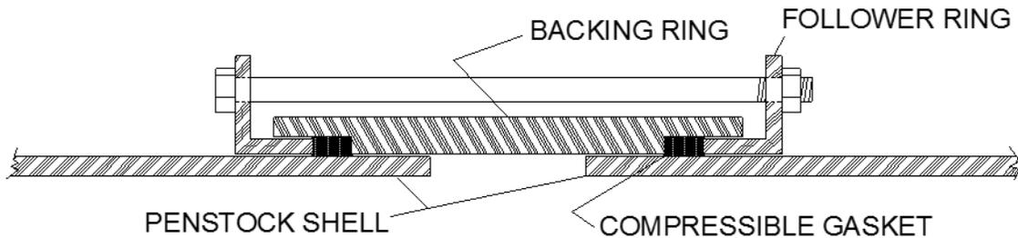
Fig. 5. Typical joint detail.
