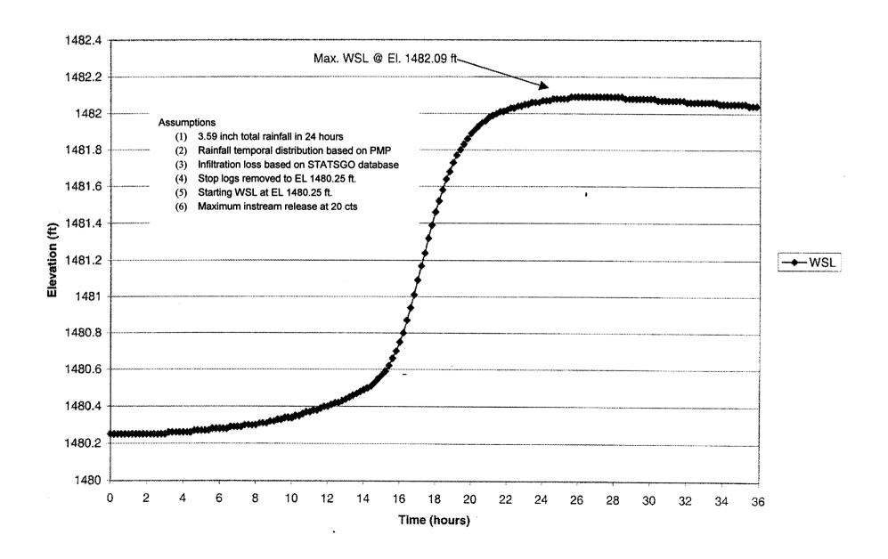
Figure 5-3 Simulated Reservoir Water Levels at Silver Lake
