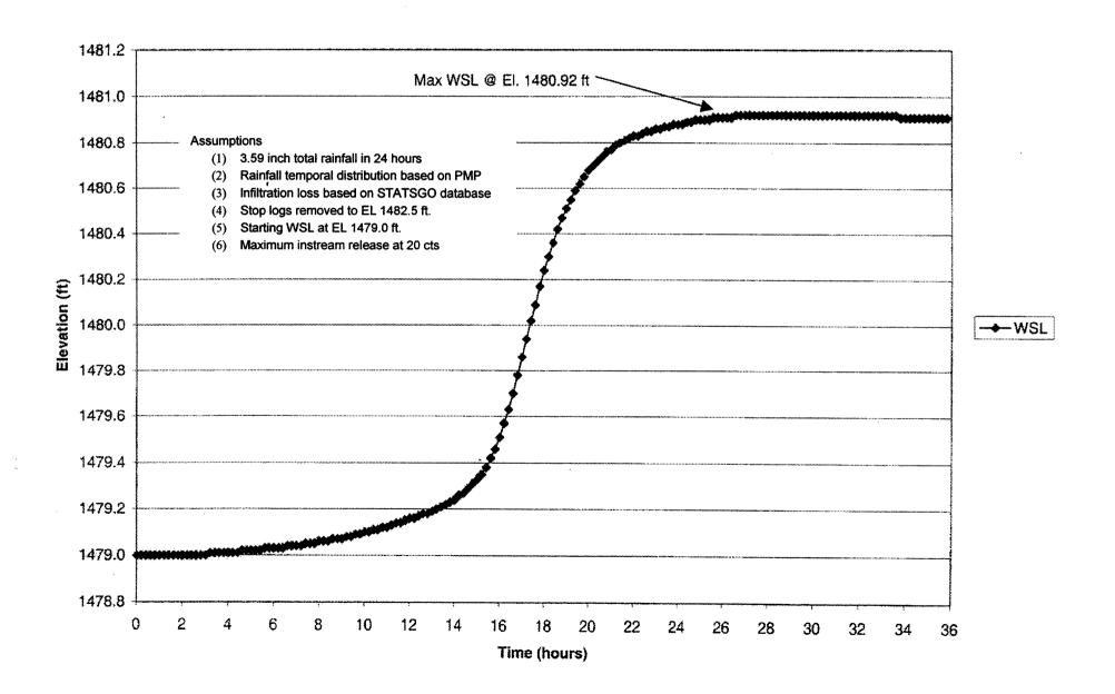
Figure 5-4 Simulated Reservoir Water Levels at Silver Lake
