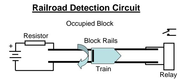
Relay at one end of block is normally energized by battery and resistor at other end of block. Locomotive or rolling stock axle in block shorts out current to relay to indicate block occupancy. Independent of Water Level Monitoring/Control Systems
