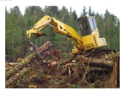
3) Dangle-head processor. Slope limited to +/-30%. Primarily delimbing, log manufacturing, and piling logs by species sort for efficient volume skidding. Production option.
