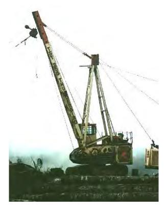
Rubber-tired self-propelled side-mounted cable yarder operating on narrow road width. Versatile configurations and mobile if safe access to tight rough terrain areas that can be yarder harvested.
