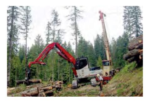
3) Yoader [aerial or ground-based]. Preferred base equipment is hydraulic heel boom log loader equipped with at least two winches. Mobile, extremely versatile, multi-tasking equipment: cable yard, log loading, shovel logging, tree pulling, slash piling. Needs minimal area for operation. Suited for cable yarding smaller timber, but can yard short length large diameter logs.
