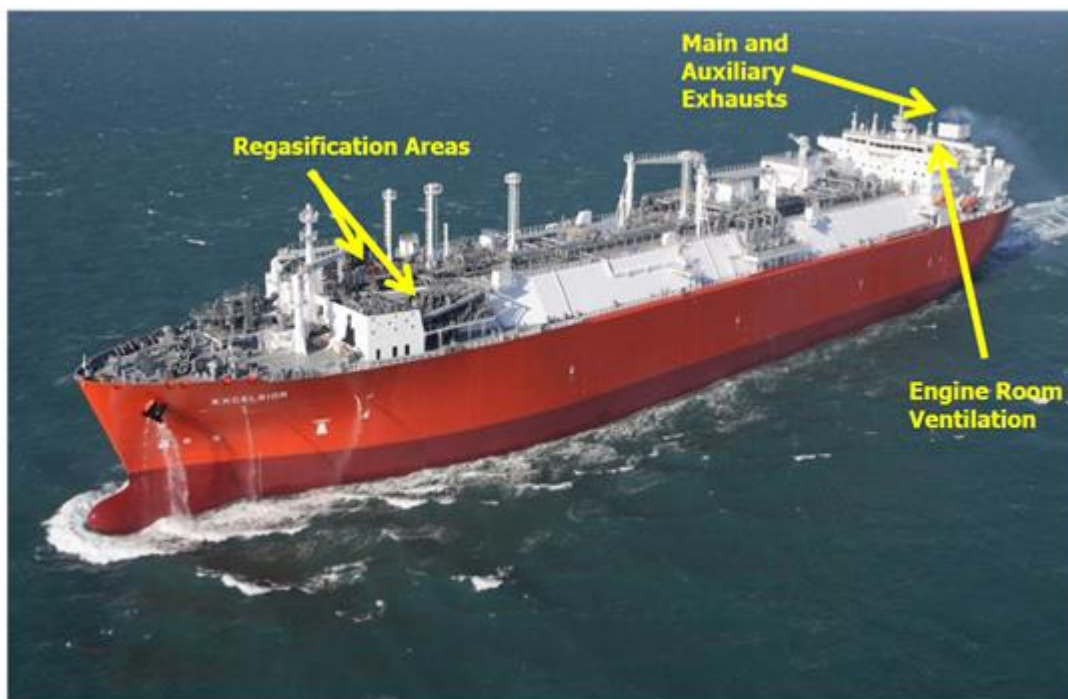
Figure 4.10.2-2: Prototype EBRV Excelsior and Areas of Principal Sound Emission
