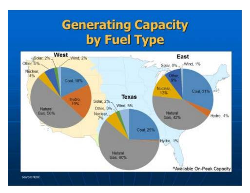
This graphic shows a breakdown of this summer's on-peak generating capacity by primary fuel type for power generation across the Western, Texas, and Eastern Interconnections.
