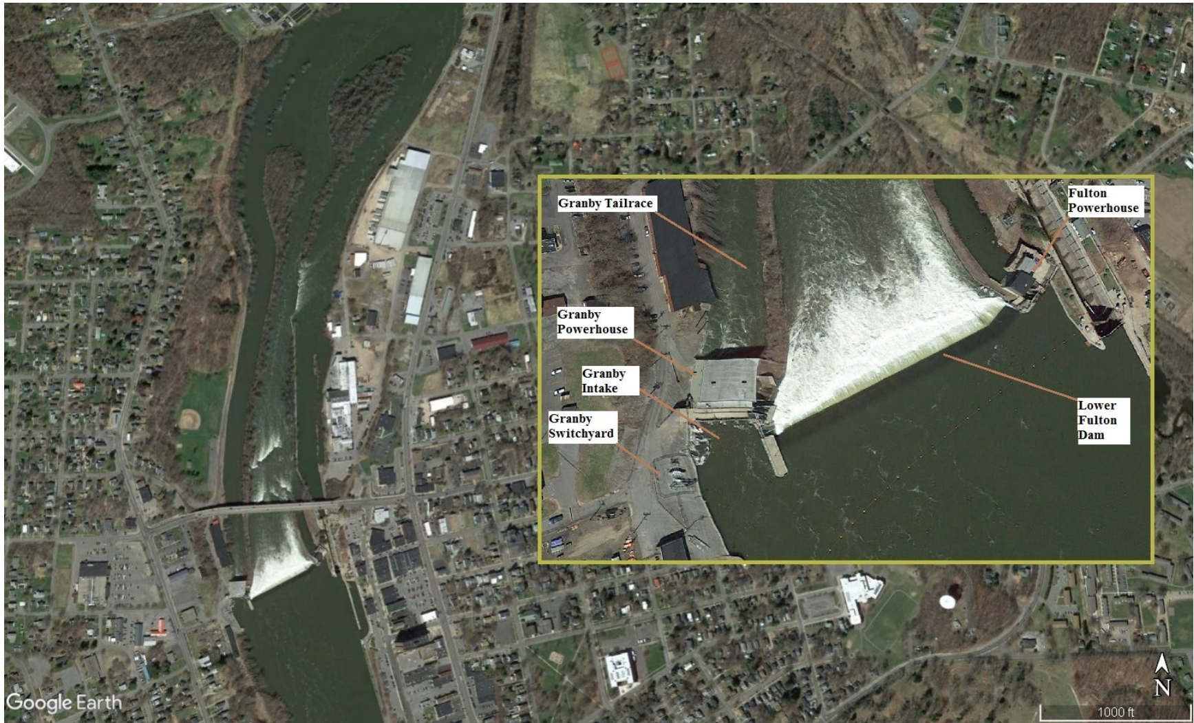
Figure 1. Location and facilities of the Granby Project (Source: Google Earth and staff).
