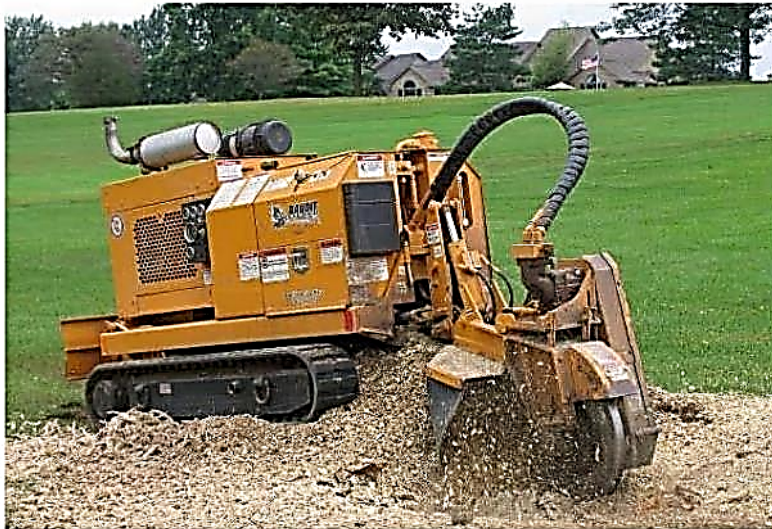
Figure 2. High-capacity stump grinder produced by the Bandit Corporation, Model 2900 SP Track. As stated by a vender's product description:
