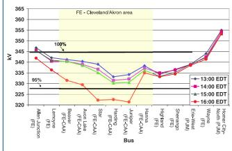
North-South 345kV Actual (Measured) Voltages Leading up to August 14th
