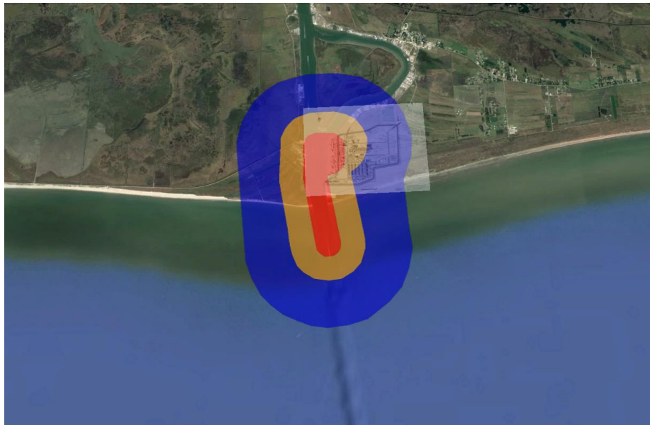
Figure 4.12.8.4-1 Accidental Hazard Zones Along LNG Vessel Route representing Zone 1 37.5kW/m 2 (red), Zone 2 5kW/m 2 (orange), and Zone 3 flammable vapor dispersion (blue)
