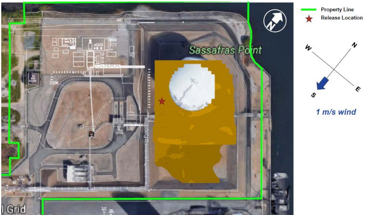
Figure 2.8.6-4 Maximum Flammable Vapor Dispersion from Scenarios LNG06 and LNG10 in the Existing LNG Storage Tank Area (using a model uncertainty factor of 2)
