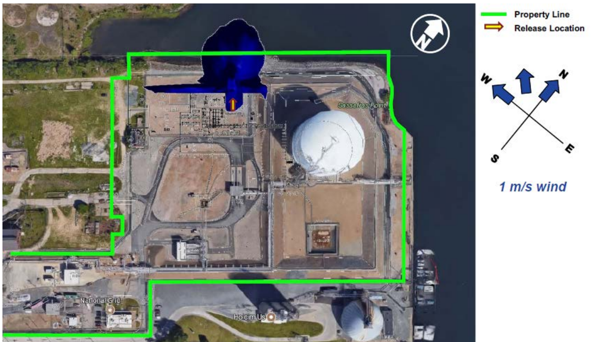
Figure 2.8.6-6 Maximum Flammable Vapor Dispersion from Regeneration Gas Knockout Drum Scenario TX01 in the Liquefaction Area (using a model uncertainty factor of 2)
