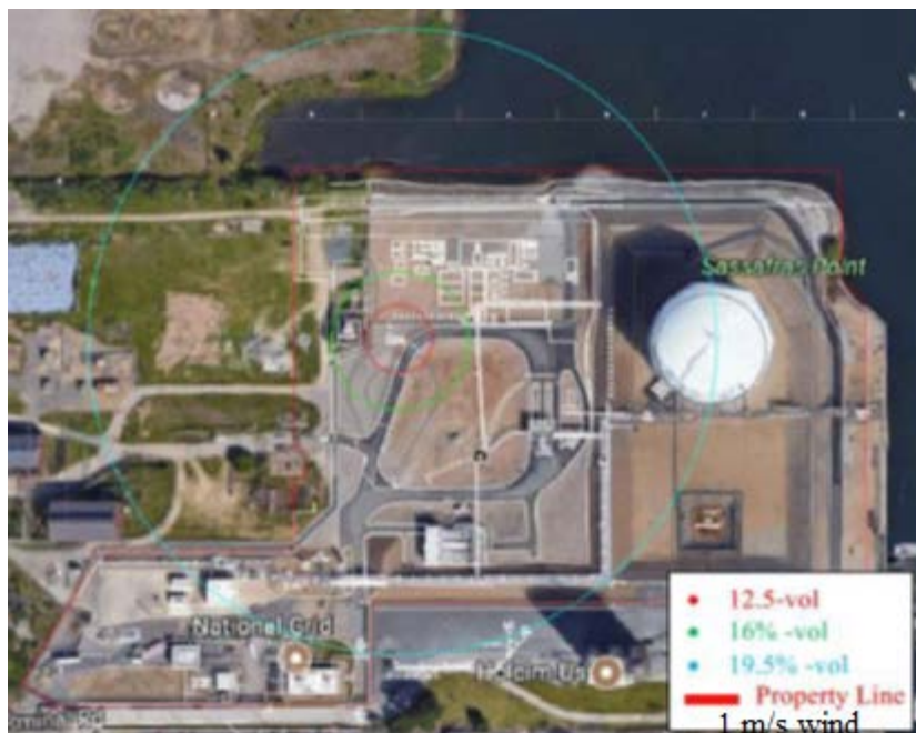
Figure 2.8.7-1 Asphyxiant Results from Liquid Nitrogen Scenario N201a (using a model uncertainty factor of 2)
