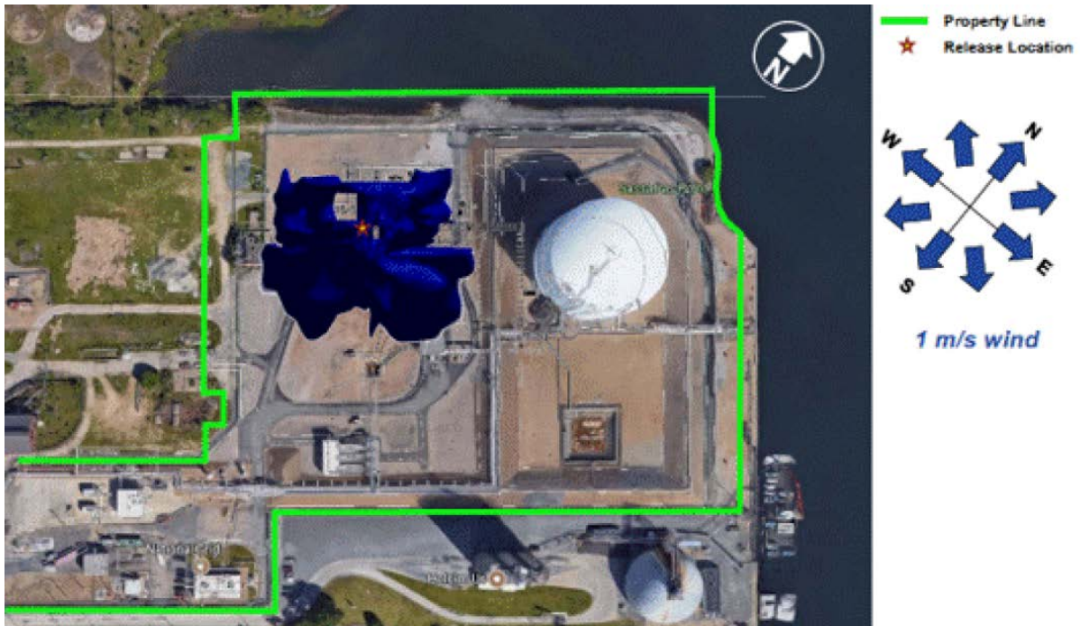
Figure 2.8.6-7 Maximum Flammable Vapor Dispersion from Heavy Hydrocarbon Scenario TX03 in the Liquefaction Area (using a model uncertainty factor of 2)
