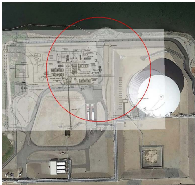
Figure 2.8.6-9 Estimated Maximum Flammable Vapor Dispersion from the Hot Oil Scenario (using a model uncertainty factor of 2 and 6 m/s wind speed)
