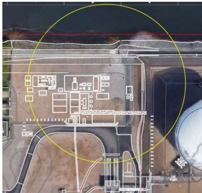
Figure 2.8.6-8 Maximum Flammable Vapor Dispersion from Natural Gas Scenario NG12 in the Liquefaction Area (using a model uncertainty factor of 2 and up to 6 m/s wind)
