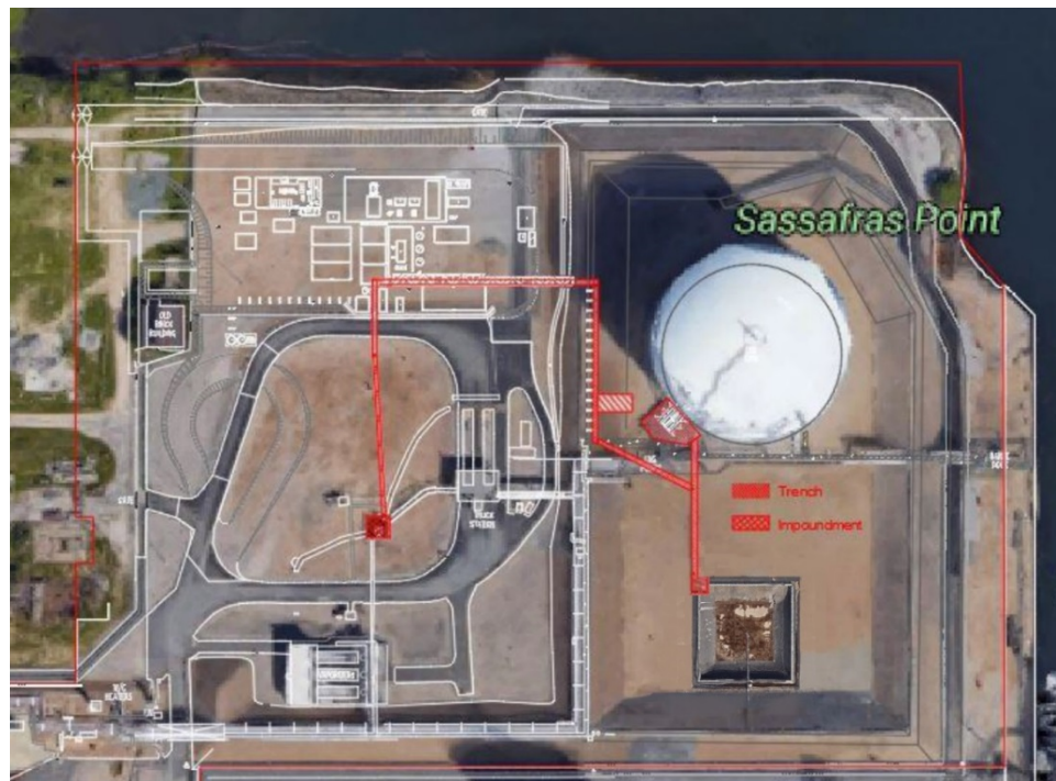
Figure 2.8.6-1 Spill Impoundment Systems
