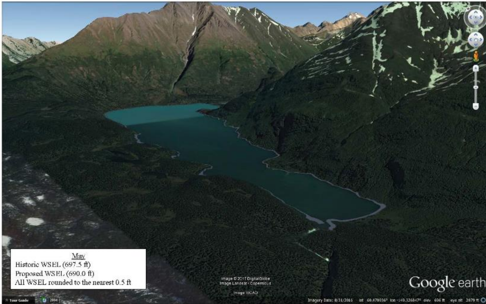
Figure 3-32. Simulations showing changes in water surface elevations associated with the project operation in May (Source: Kenai Hydro, 2017a, as modified by staff).
