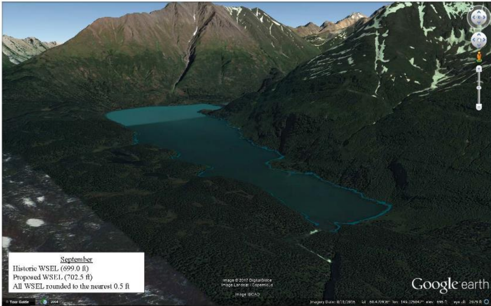
Figure 3-36. Simulations showing changes in water surface elevations associated with the project operation in September (Source: Kenai Hydro, 2017a, as modified by staff).
