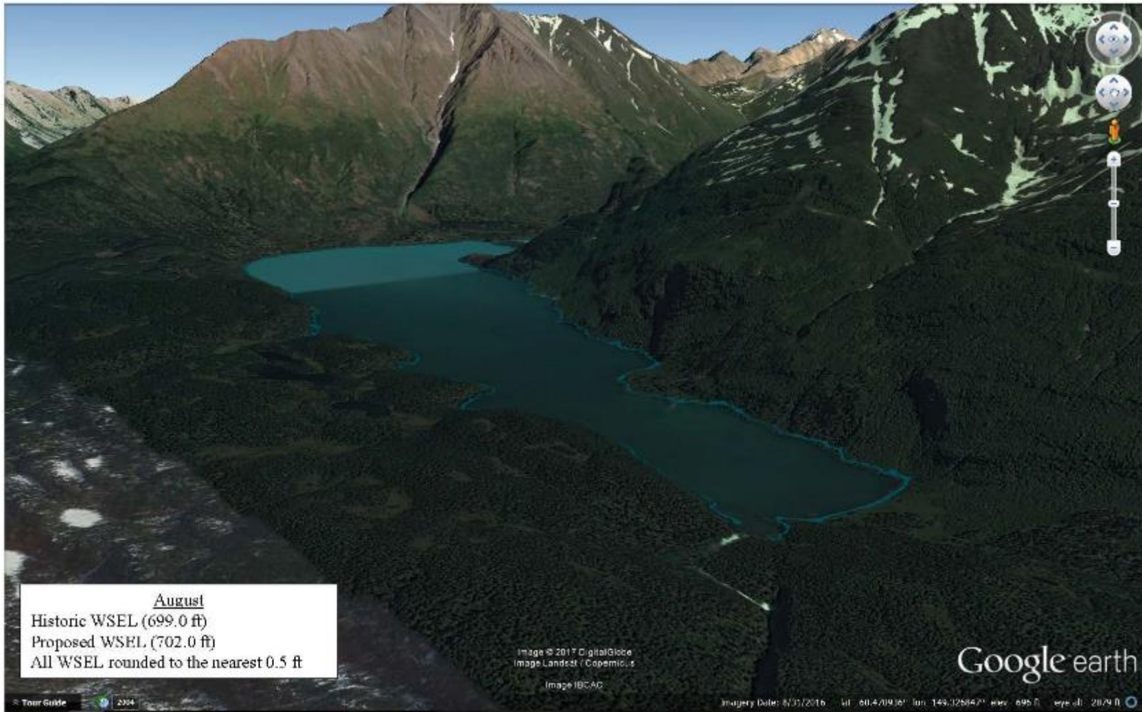
Figure 3-35. Simulations showing changes in water surface elevations associated with the project operation in August (Source: Kenai Hydro, 2017a, as modified by staff).
