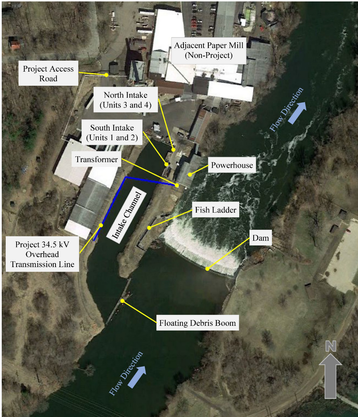
Figure 2. French Paper Project facilities (Source: Google Earth, 2019a; as modified by staff).
