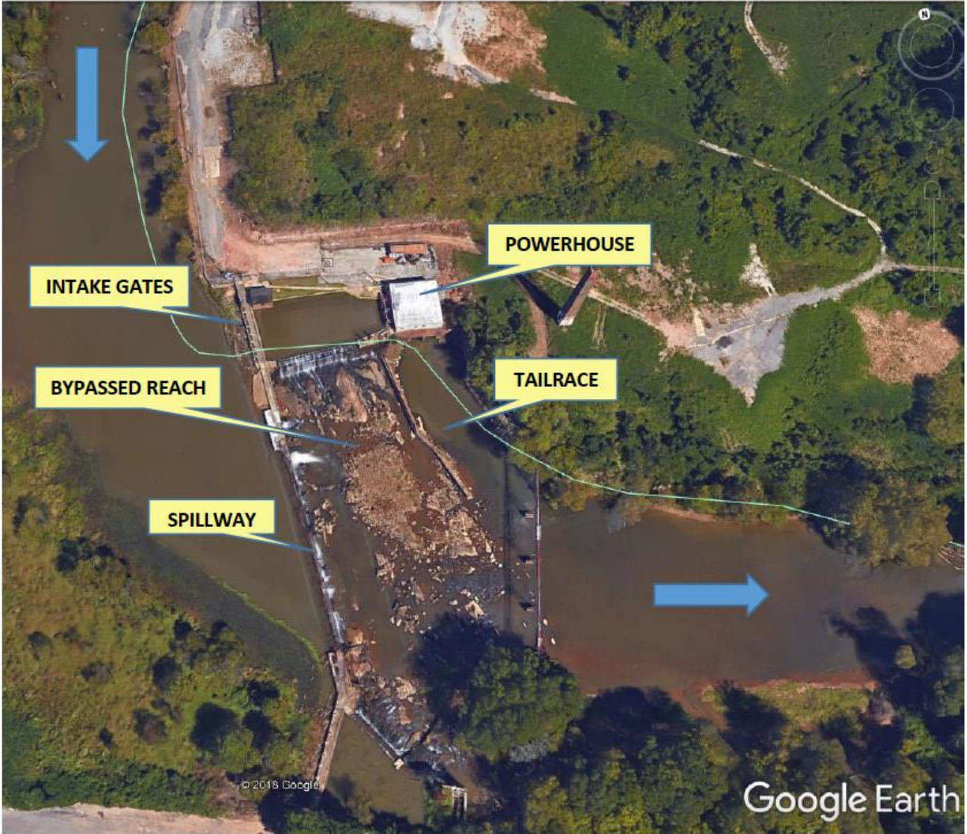
Figure 2. Project facilities for the Piedmont Project (Source: Google Earth Pro, 2018, as modified by staff).
