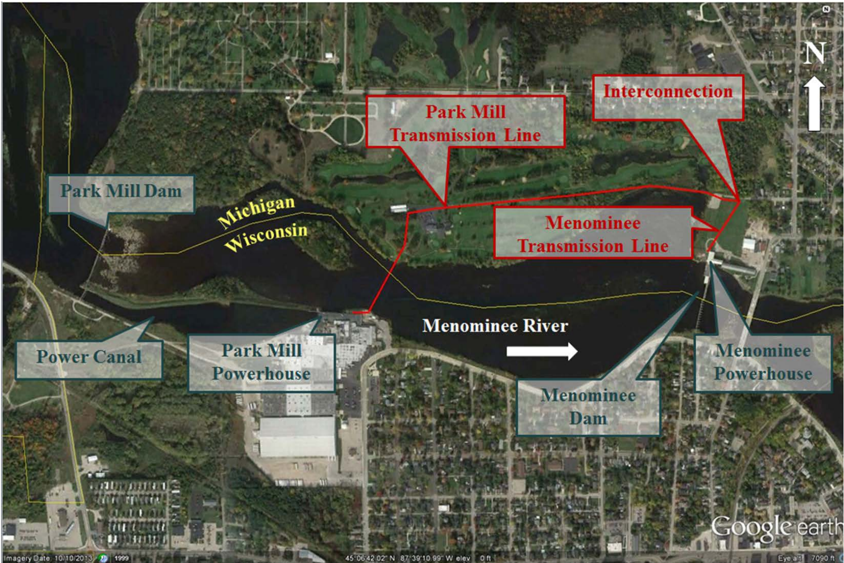
Figure 2. Project location and facilities for the Menominee and Park Mill developments (Source: Google Earth, 2016, as modified by staff).
