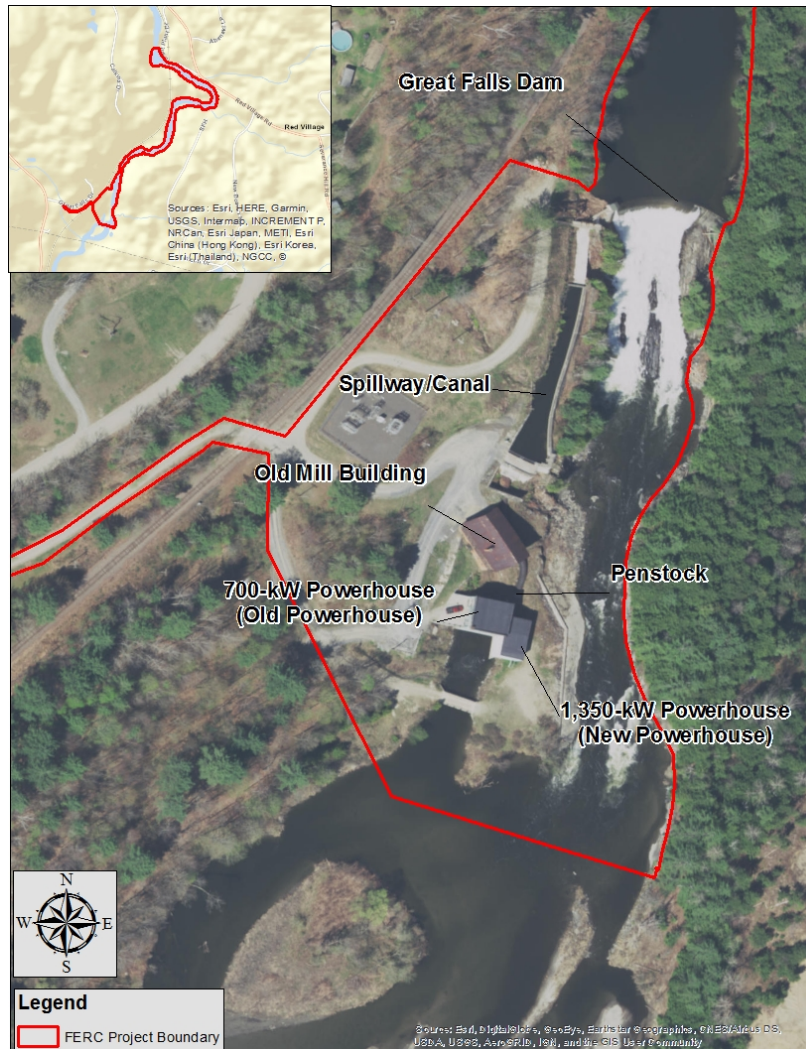
Figure 7. Contributing Resources to Great Falls Hydroelectric Station (Source: staff).
