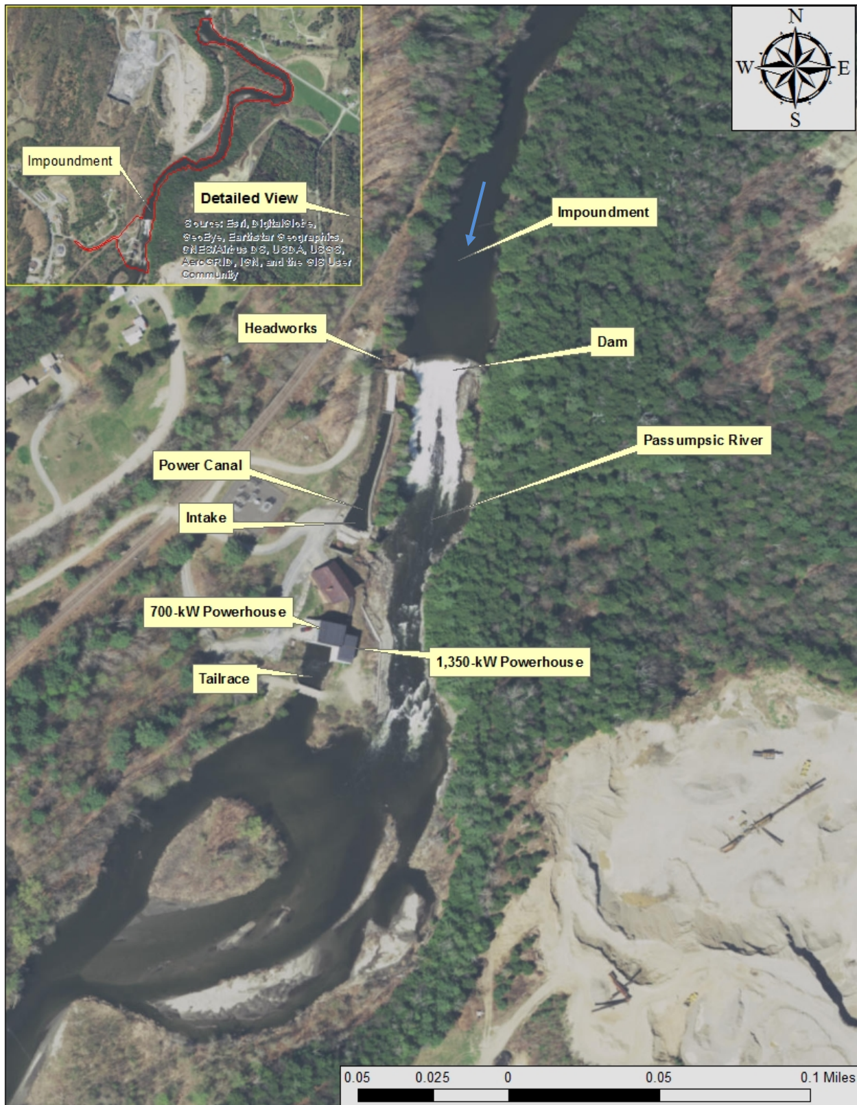
Figure 2. Great Falls Project facilities (Source: staff).
