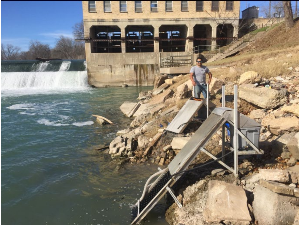
Figure 3-5. Photo of ramp traps used in the tailrace to target American eels (Source: the City, 2017)
