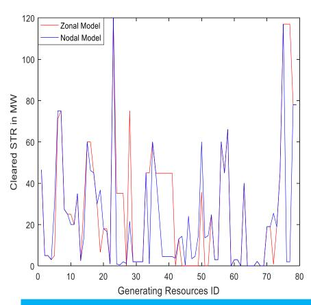
Units 76 and 77 are cleared with 117MW each and received \$257/MWh in zonal model. There zonal sensitivity is -0.23.
