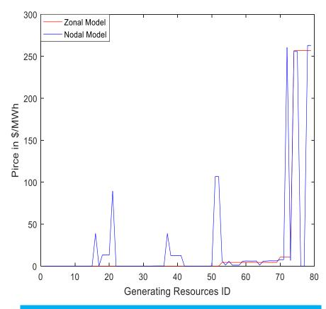
Units 76 and 77 receive \$0/MWh and are cleared with 0MW in nodal model. Their nodal sensitivities are 0.13.
